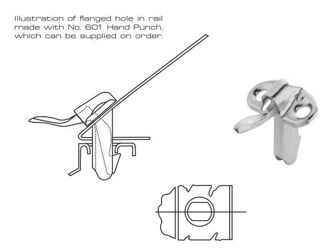
Arbor Press Unit for punching panel can also be supplied. This unit pierces two screw holes and holes for barrel of catch in one operation.
